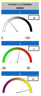
**Description of Test:** The process of making a patch isolates and agglomerates insoluble by-products associated with varnish. The color of the membrane patch provides a guideline as to the extent of varnish potential. Generally a value over 35 is considered abnormal.
