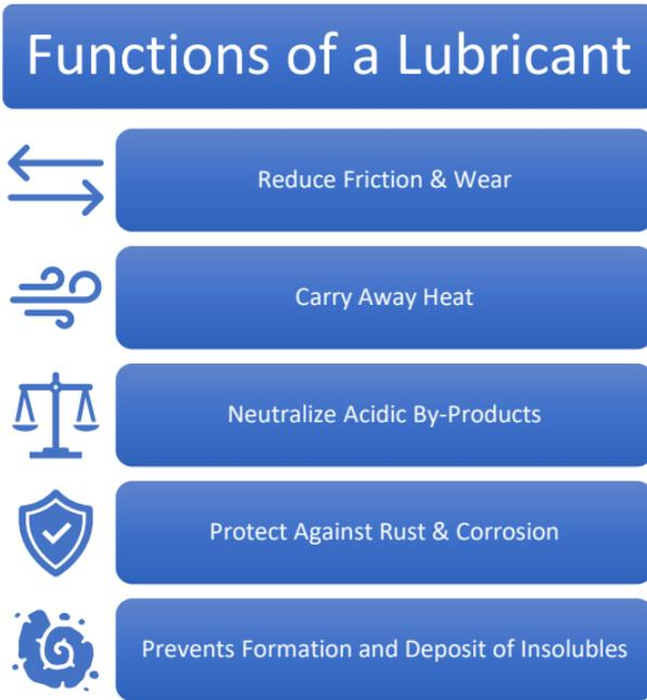
To effectively monitor how well a lubricant is working, the functions of the lubricant must be examined. The following graphic provides greater insight as to the correlation between a lubricant's function and by what method that function is tested.
