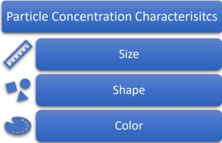
Particles are categorized based on these characteristics. Conclusions can then be drawn regarding the wear rate and health of the component that the sample was drawn from.
