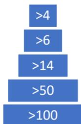
ISO Cleanliness Codes are then assigned for particles in 4, 6, and 14  $\mu\text{m}$  ranges (ISO 4406:1999). The result is reported by three numbers with a slash between them; the first number refers to particles in the >4  $\mu\text{m}$  range, the second to particles in the >6  $\mu\text{m}$  range and the third in the >14  $\mu\text{m}$  range. The lower the numbers in the ISO Cleanliness Codes, the cleaner the fluid.
