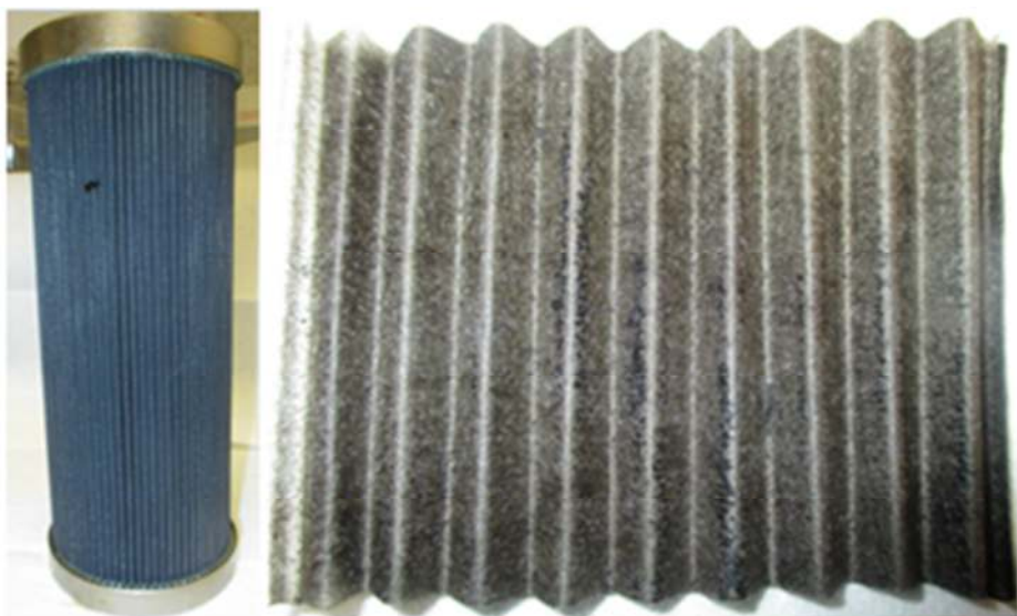
Figure 1. From left to right: filter as received, filter media selected for analysis.
