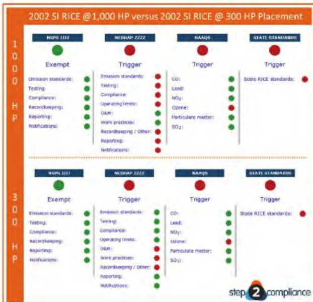
Figure 3. In this analysis, two SI RICE or natural gas engines were placed into service in 2002, with one engine above 500 horsepower and one engine below 500 hp. (Courtesy of step2compliance)
