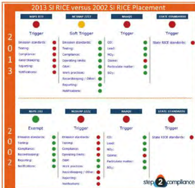
Figure 2. These results are from an applicability analysis for an SI RICE or natural gas engine placed into service in 2002 versus 2013. (Courtesy of step2compliance)
