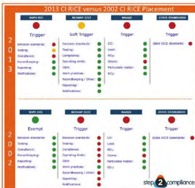
Figure 1. This graphic shows the results of a detailed applicability analysis for a stationary CI RICE or diesel engine placed into service in 2002 versus 2013. Green indicates the rules don't apply, yellow indicates something may apply, and red indicates a rule applies. (Courtesy of step2compliance)
