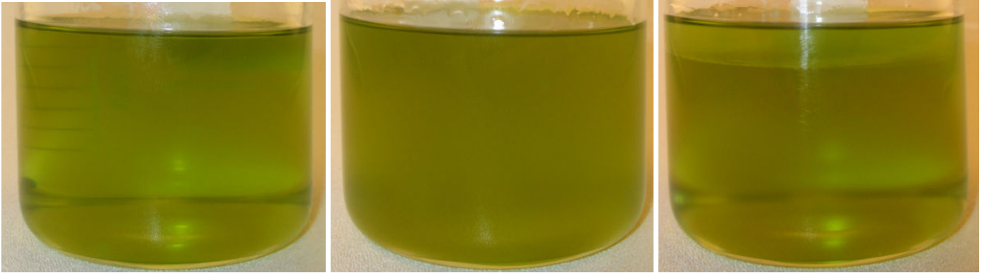
Figure 4 Sullube 32/Quinsyn Plus after heating, after one hour cool down, and after overnight at room temperature.
